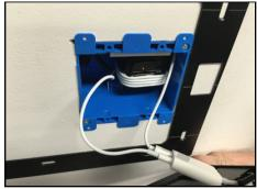
**3.** Plug the USB adapter into the iPad and insert the iPad into the Surface Mount.
